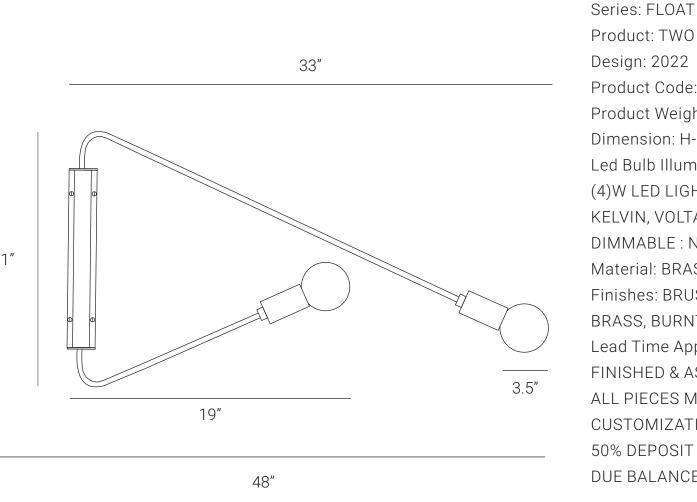
Product: TWO ARM WALL SCONCE Design: 2022 Product Code: LSETAWS Product Weight: 4KG Dimension: H-21", W-33", D-48" Led Bulb Illumination: SOCKET BASE-E27, (4)W LED LIGHT, COLOR TEMPERATURE, (3000) KELVIN, VOLTAGE (220-240), CE APPROVED DIMMABLE : NO Material: BRASS Finishes: BRUSHED BRASS, RAW BRASS, AGED BRASS, BURNT BRASS Lead Time Approx: 5-6 WEEKS **FINISHED & ASSEMBLED BY HAND** ALL PIECES MADE TO ORDER CUSTOMIZATION AVAILABLE 50% DEPOSIT IT REQUIRED DUF BALANCE PRIOR TO SHIPPING
